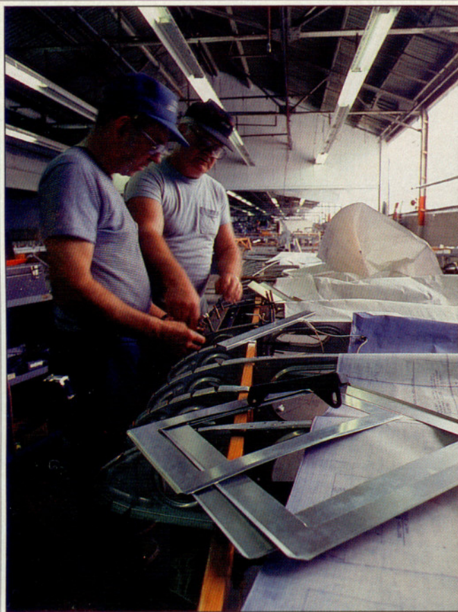
The Taylorcraft has been given many improvements over the years, such as wider doors and flaps (bottom), but the manufacturing process is just like the old days: wooden spars, aluminum ribs, and lots of careful handwork.
