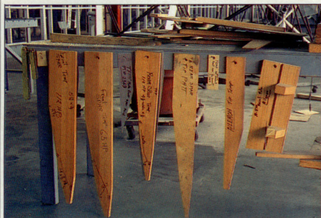
The Taylorcraft has been given many improvements over the years, such as wider doors and flaps (bottom), but the manufacturing process is just like the old days: wooden spars, aluminum ribs, and lots of careful handwork.
